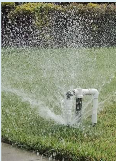
A pipe constantly under pressure burst, draining thousands of gallons before being shut off.
